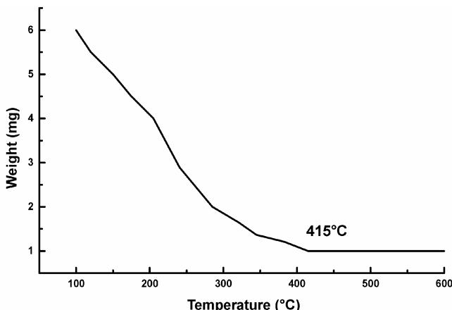
**Figure 1.** TGA result of the film obtained spraying the neodecanoates solution used to synthesize Y-123 samples.
