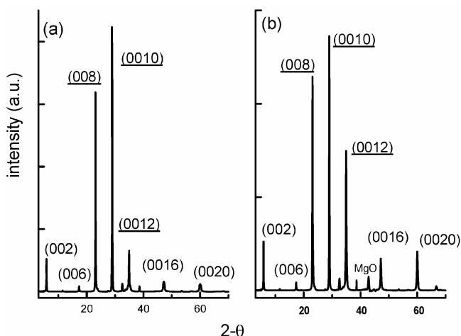
**Figure 5.** XRD spectra of BSCCO samples obtained on Ag (a) and MgO (b) substrates starting from neodecanoates.
