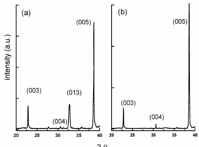
**Figure 4.** XRD spectra of YBCO samples obtained on Ag (a) and MgO (b) substrates starting from neodecanoates.
