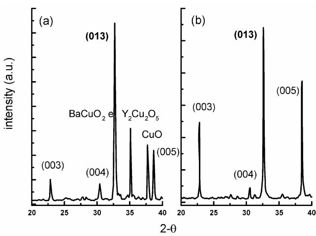
**Figure 3.** XRD spectra of samples of YBCO obtained on  $\text{Al}_2\text{O}_3$  substrate starting from 2-ethyllesanoates (a) and neodecanoates (b).
