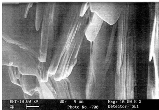
**Figure 6.** SEM pictures of Bi-2212 film obtained on MgO.
